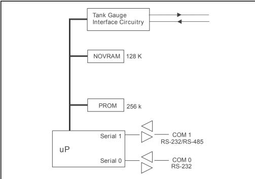
The heart of the TankGate is an Intel 80C188EB microprocessor operating at 18.432 MHz. Designed specifically for real-time embedded applications, the  $\mu P$  includes timer/counters, an interrupt controller, and chip-select circuitry. It also includes 2 serial channels that are designated as COM0 and COM1.
